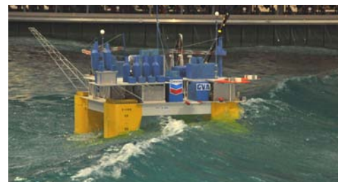
Semi model in the Ocean Basin, 100-year storm.
