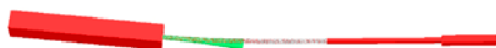
Figure 2. Numerical model of the full-scale tests. The tower to which the green bellmouth is attached is the red section on the left side. Rotation is applied on the right-hand side of the tower.
